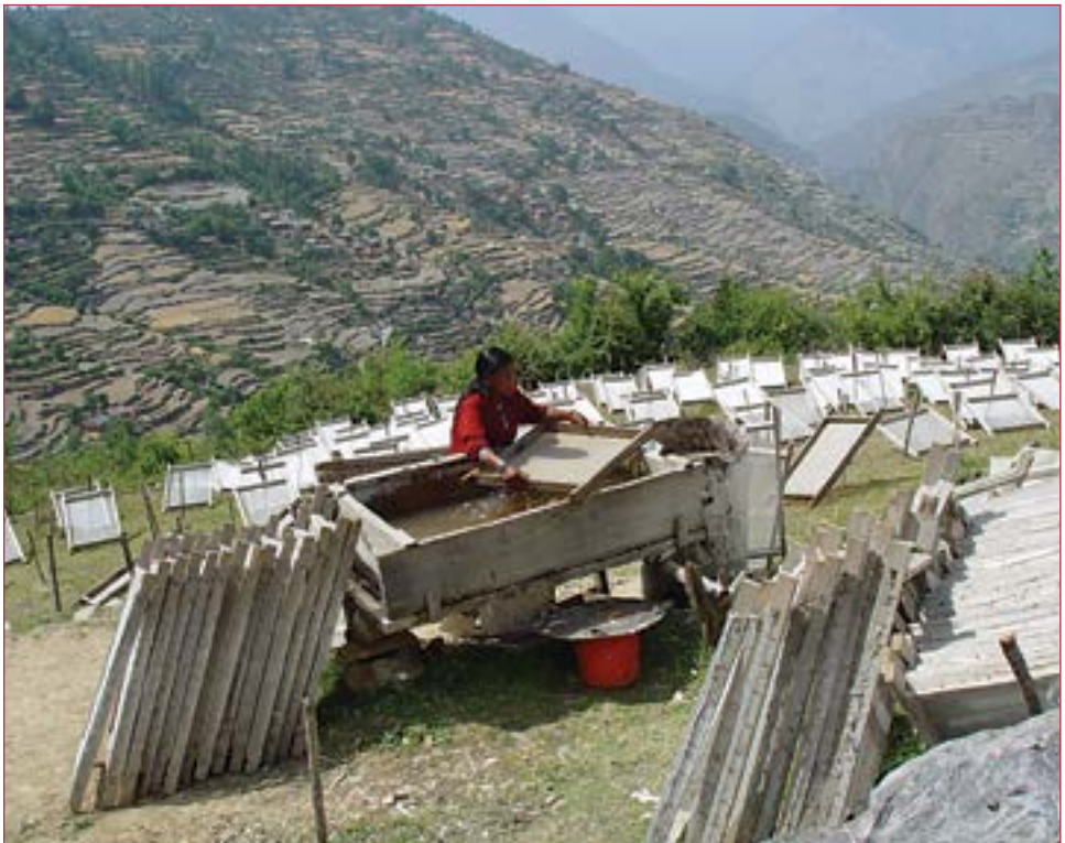
Handmade paper made from lokta pulp. The paper sheets are dried in the sun on wooden frames
