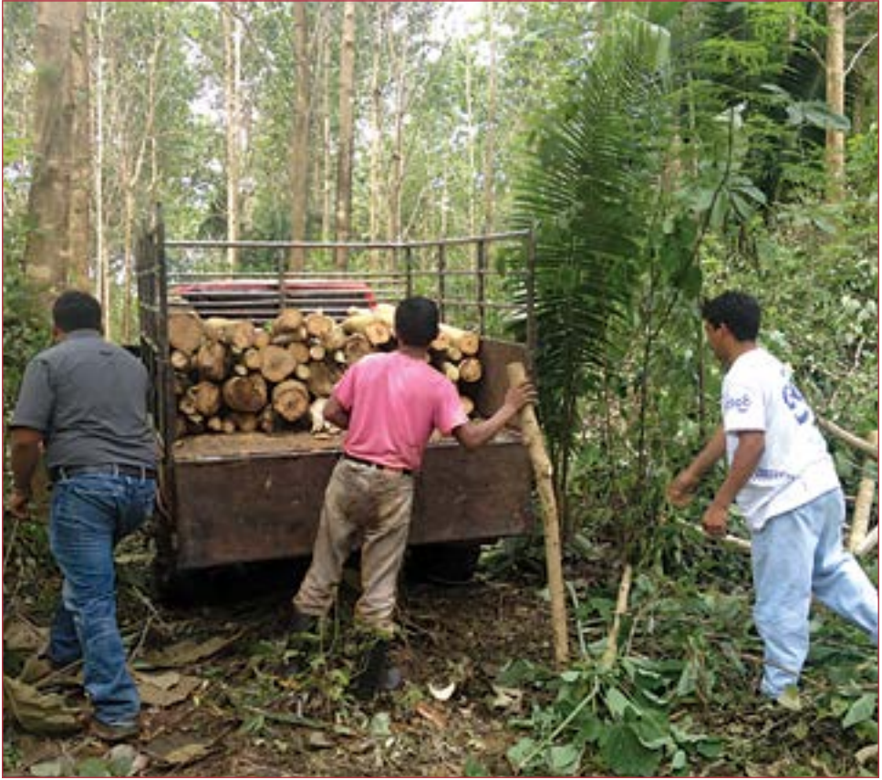
Skidding (moving the felled timber to a landing site using 4x4 pick-up trucks) and vehicle loading are done by hand
