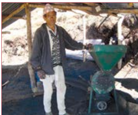
The electric grinder used to produce char powder which is then mixed with clay and moulded into briquettes
