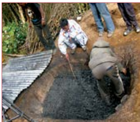
Burning of raw material into char using the pit method before transporting it to the briquette-making facilities
