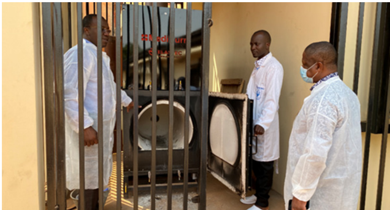
Dr. Abel Wade, LANAVET Director, shows Mr. Gordon Okpu, CDC GHSA coordinator, the incinerator funded by DTRA's investment in GHSA-Cameroon. This incinerator is one of few in Cameroon able to properly destroy infected large animal corpses. Photo: Daphne Moffett/CDC
